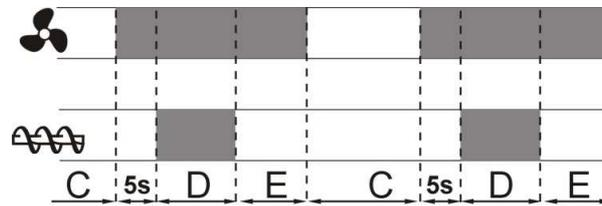
Fig. 9 Cycles of fan and feeder operation in SUPERVISION mode; C – *Feeder Interval - Superv.*, D – *Feeding Time-Superv.*, E – *Blow-in operation extending- Superv.*
